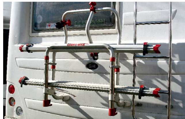
A central rear door on your motorhome (right) will prevent the fitting and use of a regular bike rack (above), so you might have to consider mounting the rack on a custom-built hinged frame, instead
