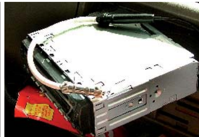
A standard-sized radio, otherwise known as a single 'DIN', is 50mm high. Those which are 100mm high are called 'Double DIN'
