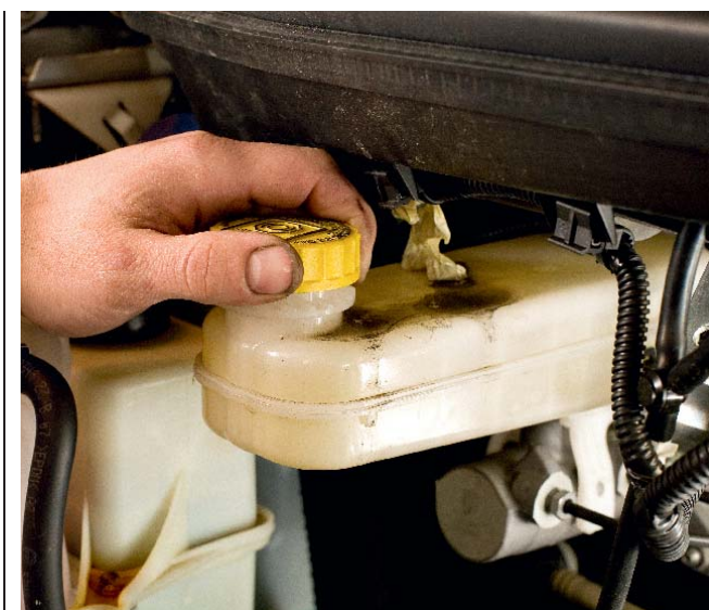
Always make sure that your engine is completely cold before removing the coolant tank cap, or the water within may boil up
