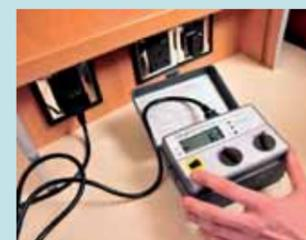
The next test was to make sure the electrical trip switch was working effectively. Lee's RCD reader sent an electrical surge through the system to measure the time it took for the trip to work. Anything over 40 milliseconds (0.040 seconds) means the switch would need replacing.
