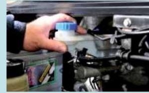
Still under the bonnet, the fluid levels were checked – this included coolant, washer bottle water and brake fluid – making sure that each had the correct levels for proper functioning.
