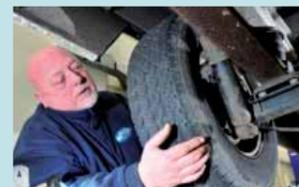
The next test was on the wheel bearings. Dave pulled each wheel top and bottom, to check for any play in the hub.
