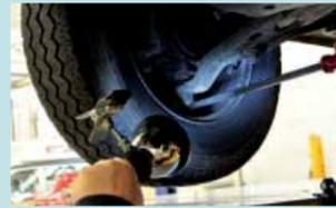
Next, the 'van was lifted on ramps and jacked up ready for the inspections underneath. Checking inside the wheel, Dave examined the ball joints.
