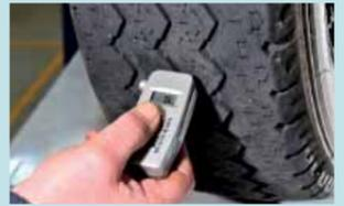
Using a special digital tread-depth gauge, Dave was able to get a highly accurate reading to show whether or not the treads were in a legal condition.
