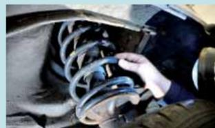
The front and rear suspension springs and struts were examined to check they are holding up, not leaking any fluids and that they are able to support the weight of the 'van, with no excessive bounce.
