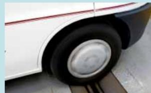
On a rolling road, Dave tested the brakes and then carried out an engine emissions test.
