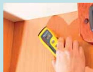
Inside the Auto-Sleeper, Lee checked for damp by running his meter around the various panels. He told me that a reading above 15 per cent would be considered severe, indicating that the offending areas were in need of attention.
