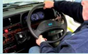
The Lifestyle's steering wheel was wiggled backwards and forwards to make sure that there was no play in the steering column, and that it was therefore attached and working correctly.
