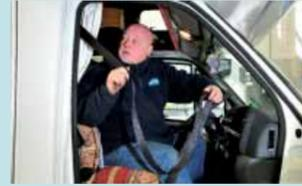
Dave (pictured here) first checked the interior. He made sure the front seat belts were secure and undamaged, and similarly the seatbelts on the rear travel seats.
