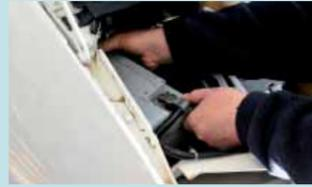
Dave then tested the engine battery for the correct voltages, and made sure that it was not leaking acid, and that there was no danger of anything catching and shorting out.
