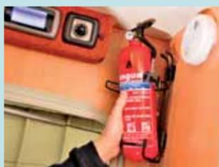
The fire extinguisher was taken from its mounting to make sure it was free, and fully charged, just in case it is ever needed. (An important check for us all. See G. O'Neill's letter on page 29)
