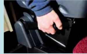
The next check was on the handbrake: Dave pulled it up hard to make sure that it locked properly and that there was no slack in the cable.
