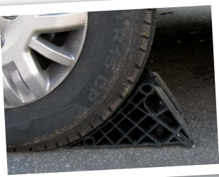
Left Check the wheels of your 'van and release the handbrake to prevent brake seizure later Above Before storing your 'van over the winter, write yourself a 'To do' list
