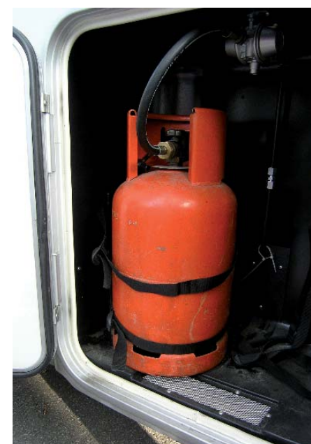
Propane is better than butane in cold weather but you will need to change the 'pigtail' connector (circled)
