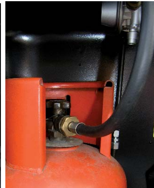
Propane is better than butane in cold weather but you will need to change the 'pigtail' connector (circled)
