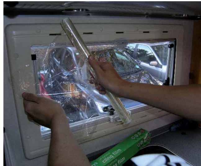
Stretching a length of cling film over your motorhome's habitation window frames is a cost-friendly alternative to double-glazing
