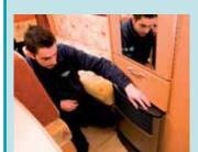
Lee also made sure that the vehicle's gas heater was working properly with blue flames, and no blockages that otherwise might lead to the formation of carbon monoxide.
