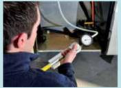
Lee (*pictured here*) went around the outside of the 'van and inspected the gas lines, testing the pressures: if they dropped, it would indicate a leak somewhere in the system.
