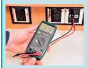
Because this Auto-Sleeper has a sealed leisure battery box, Lee checked the voltage through an auxiliary socket and received a perfect fully-charged reading of more than 14 volts.
