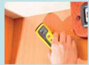
Inside the Auto-Sleeper, Lee checked for damp by running his meter around the various panels. He told me that a reading above 15 per cent would be considered severe, indicating that the offending areas were in need of attention.
